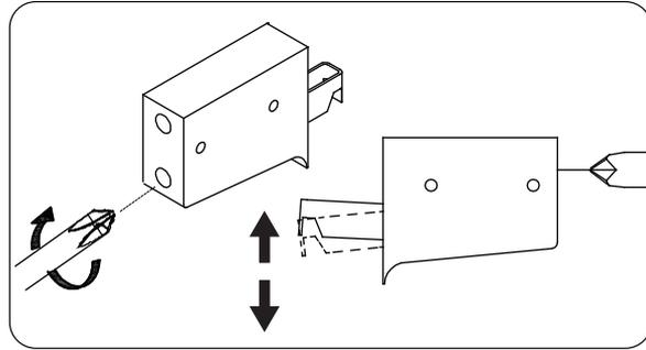
iii. When unit is hanging on the brackets, tighten lower screws clockwise, so clamping unit to wall - do not over-tighten.
