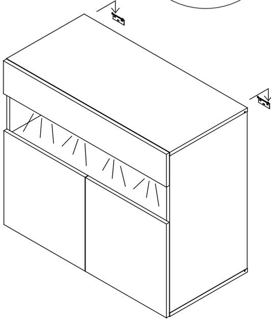
ii. With help, hang the cabinet onto the metal wall brackets by carefully aligning the end panels so they just miss the ends of the brackets. Turn upper screw(s) on either side until unit is horizontal.
