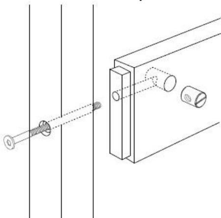
The barrel nut must be inline with the bolt. After insertion the bolt will thread through the nut to secure.
