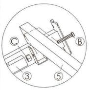
2.1 Place the width bars [5] into their corresponding "U" shaped brackets on the side rails [3]. Tightly secure the width bar [5] using the 1/4"x40mm screw[B] and nut[C].
