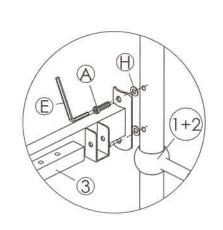
Attach the side rails [3] to the headboard [1] & footboard [2] with M8 x 25mm screws[A] & Plastic washer.
