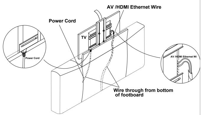
Place the wire cable through the Cable Management Caps to prevent any damage to the wire cable (eg.other power cord) when TV Lift Mechanism is operating. Make sure the wire cables are long enough to let the TV Lift Mechanism move freely.
