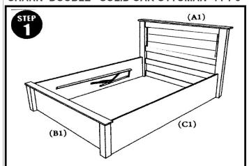
Attached the side rail (C1) to the headboard (A1) with bolt (S1). Secure into position using the supplied allen key to tighten Repeat to attach to the footboard (B1)
