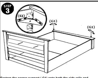
Fastern the corner support ( G1) onto both the side rails and footboard with bolt (S2)
