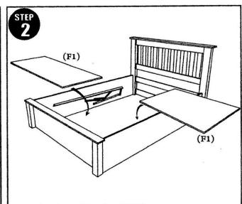
Place the plywood base board (F1) into storage area (as shown).
