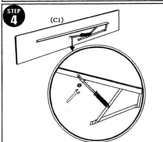
Attach the pre-fitted gas spring to the side rail brackets with pre-fitted bolt.
