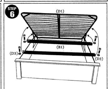
Attach the horizontal support bar (E1), under the metal frame (D1) (as shown) with mechanism (D3).
