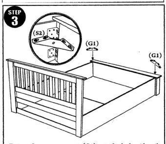
Fastern the corner support (G1) onto both the side rails and footboard with bolt (S2).
