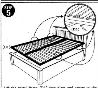
Lift the metal frame (D1) into place and secure to the mechanism (D2) on the side rail.
