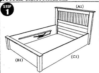
Attach the side rails(C1) to the headboard(A1) with bolts(S1). Secure into position using the supplied allen key to tighen.
