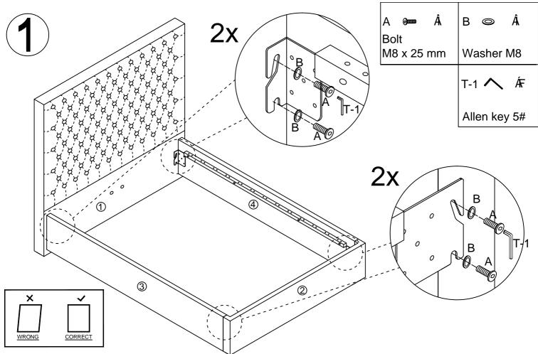
ATTENTION: Please use washers following Assembly Instruction and tighten all bolts before using. Otherwise it would make the central support rail and legs vulnerable, the bed may collapse.
