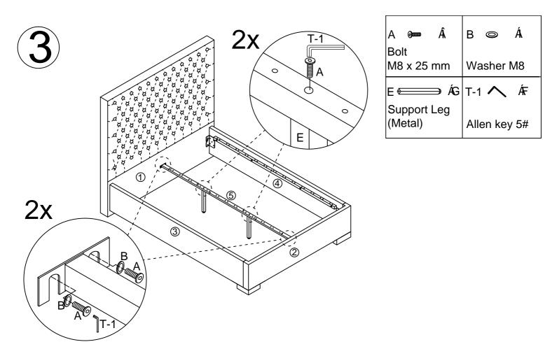
**ATTENTION:** After central rail and support legs being assembled, rotate adjustable feet to make support legs 10mm away from the floor. Support legs would touch the floor when a mattress is put on the base.
