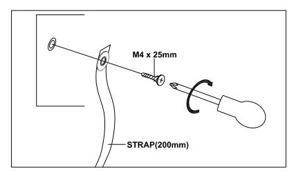
**NOTE**: Wall fixing are not supplied with this product as different wall materials require different types of fixing devices (such as Rawl plugs on bricks wall). You must use fixing devices suitable for the type of wall you intend to mount this product to. Please ensure that the head of any screw used has a diameter greater than the diameter of the mounting hole on the product and that the fixing is safe and secure before use.
