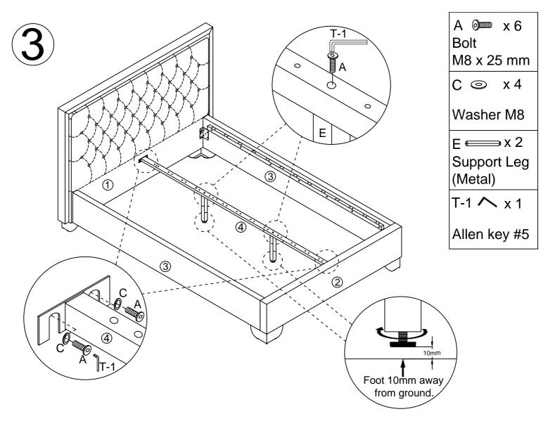
ATTENTION: After central rail and support legs being assembled, rotate adjustable feet to make support legs 10mm away from the floor. Support legs would touch the floor when a mattress is put on the base.
