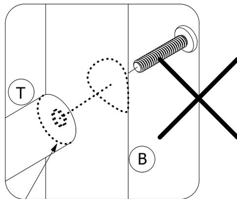
**Incorrect:** Part T NOT penetrating through Part A, B, C & D.
