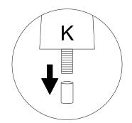
NOTE: remove the protective cap on foot (K) before beginning assembly.
