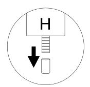
NOTE: remove the protective cap on support leg (H) before beginning assembly.
