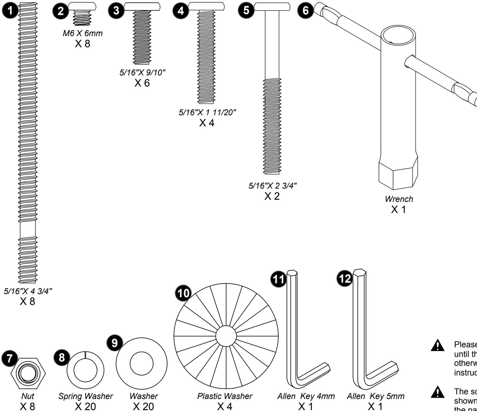
**!** Please do not completely tighten all the hardware, until the entire assembly is complete, unless otherwise indicated in the step-by-step instructions.
